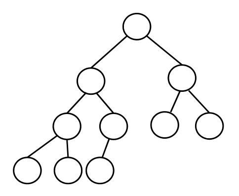
A *complete binary tree* is a binary tree of height h such that every level less than h is full and all nodes at level h are as far to the left as possible
