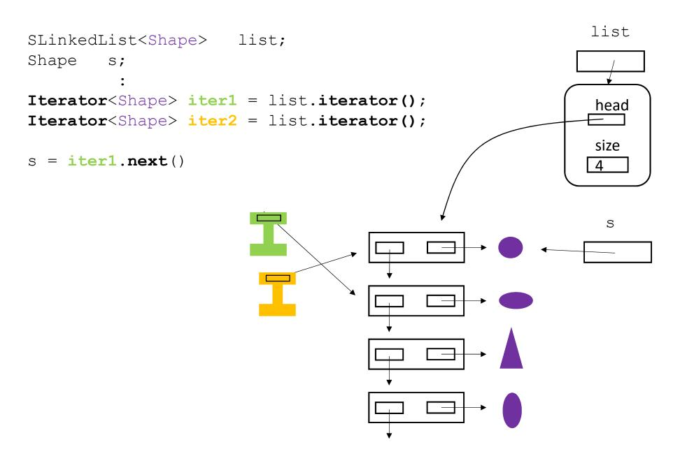
The iterators iterate over SNodes, not Shapes. The next () method returns a reference to a Shape.
