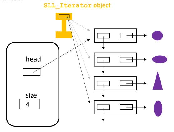
The SLL\_Iterator object will iterate through the nodes and return the element referenced by each node.
