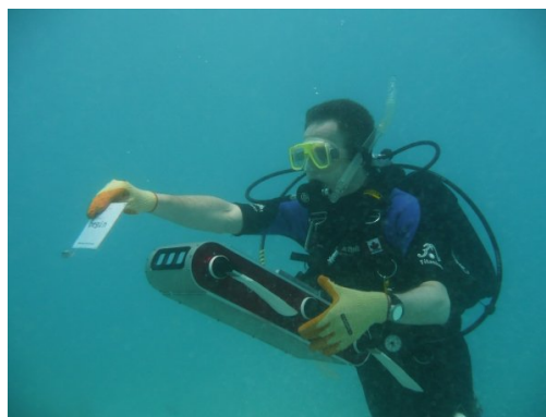
Figure 1. The Aqua robot operating tetherlessly on visual stimuli: a scuba diver starting the robot by showing a tag.
