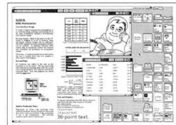
Figure 1. ViewPoint screen image. Star's bitmapped display, once unique in the marketplace, is now much more common. Such a display permits WYSIWYG editing, display of proportionally spaced fonts, integrated text and graphics, and graphical user interfaces.
