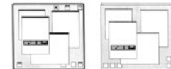
Figure 3. Visual order and user focus. The large amount of contrast present on the screen of many window systems (left screen) makes it difficult to focus on the relevant information. The selection should be the user's main focus: it is the object of the next operation. The right screen shows how Star/ViewPoint's screen design focuses attention on the selection.
