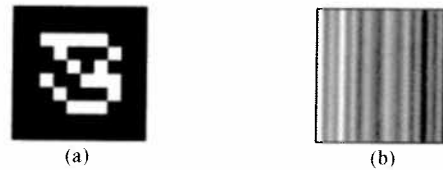
Fig. 1. a) An ARTag marker encodes data using black and white squares; b) A Fourier Tag marker embeds data into the frequency spectrum of the image.
