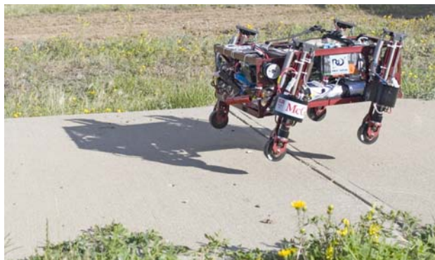
Fig. 1. The PAW robot bounding outdoors on concrete using active wheel control . Photo courtesy of Defence R&D Canada.
