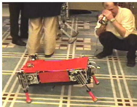
Figure 1. Scout II: A high performance, autonomous four-legged robot, running during a demonstration in Kyoto, Japan.
