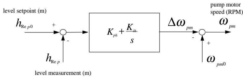
**Figure 2: Repulper tank level PI controller**
