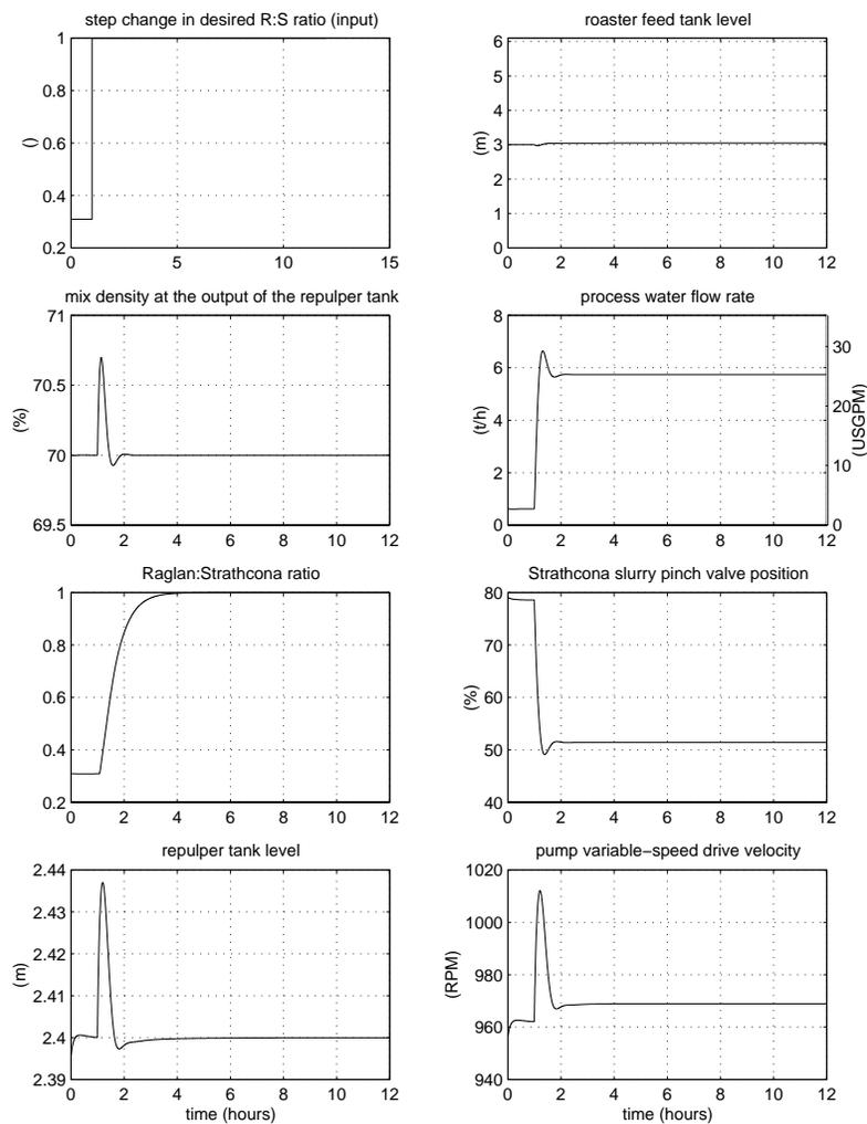
Figure 7: Response to a +0.691 step change in R:S ratio setpoint
