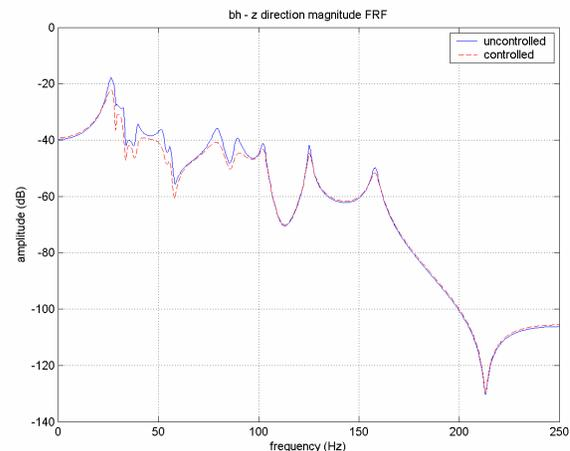
Figure 9 – bh, z direction closed-loop dB attenuation on randomized model
