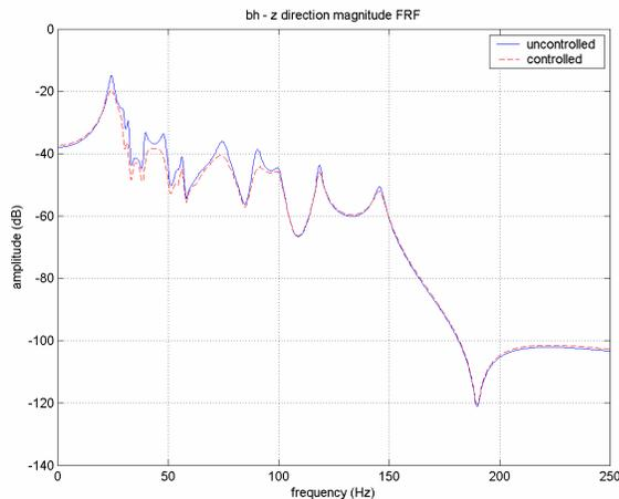
Figure 8 - bh, z direction closed-loop dB attenuation
