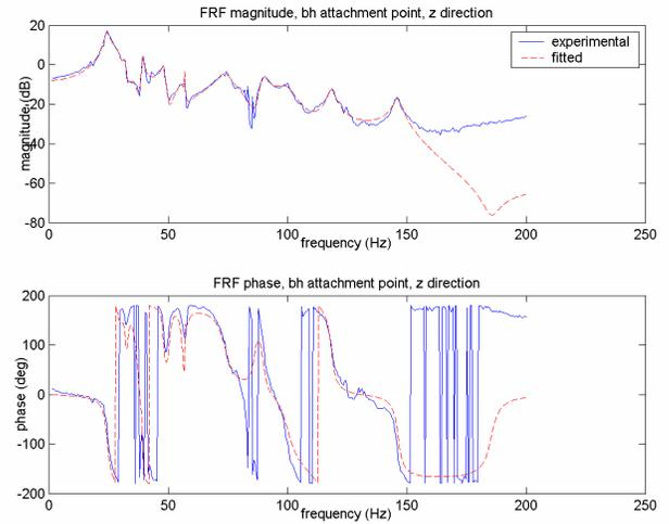
Figure 6 - Fit performed on the FRF taken at bh, z direction
