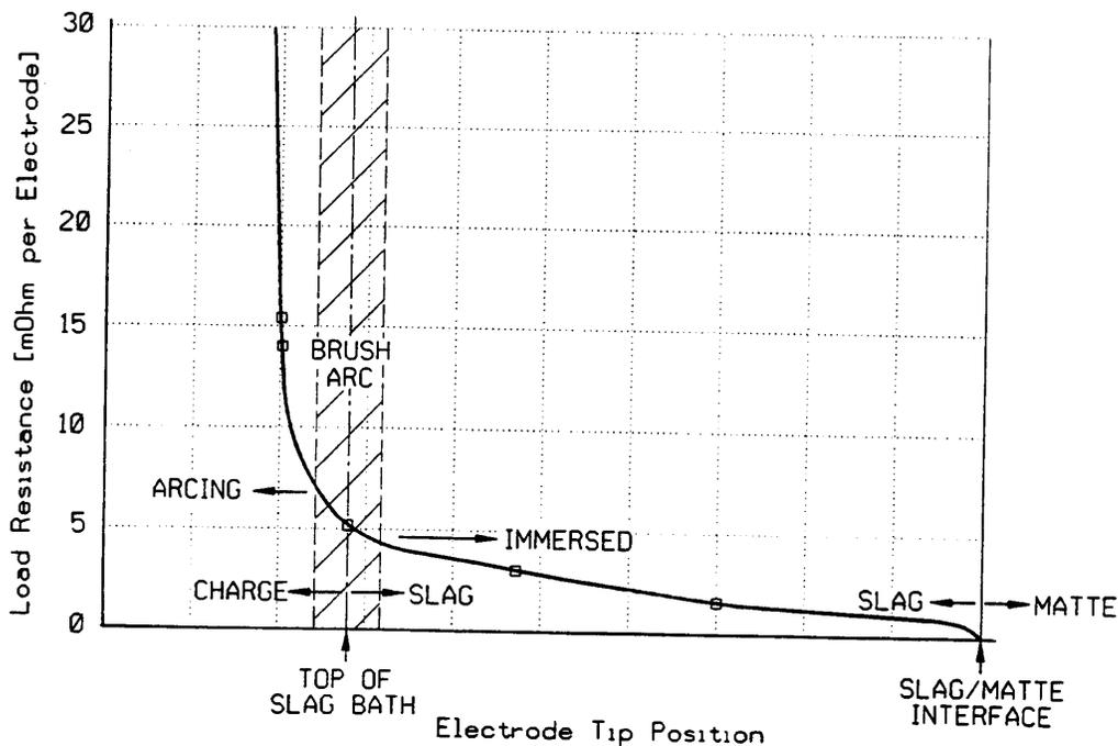
Figure 6: Electrode resistance versus electrode immersion
