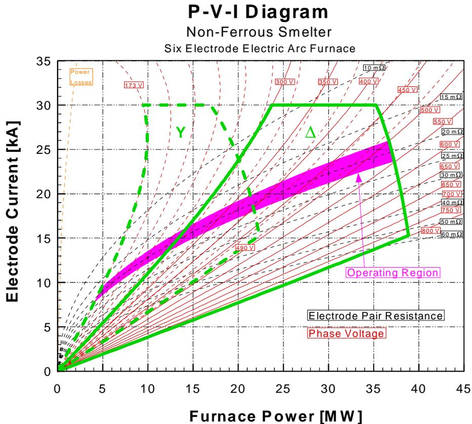
Figure 4: PVI chart for a six-electrode furnace
