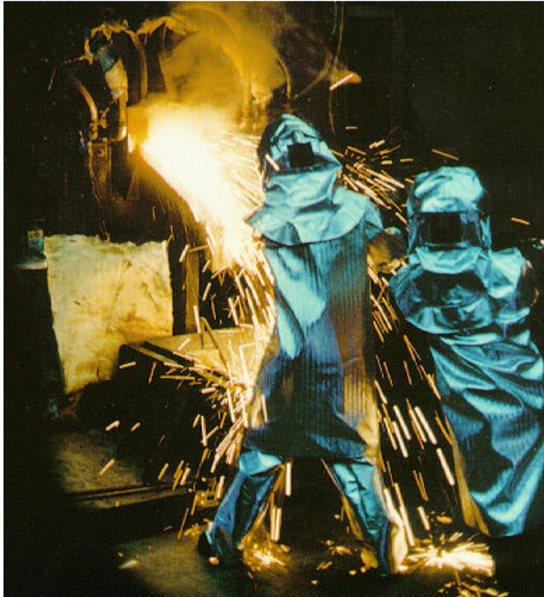
**Figure 1: Matte tapping on an experimental DC furnace**
