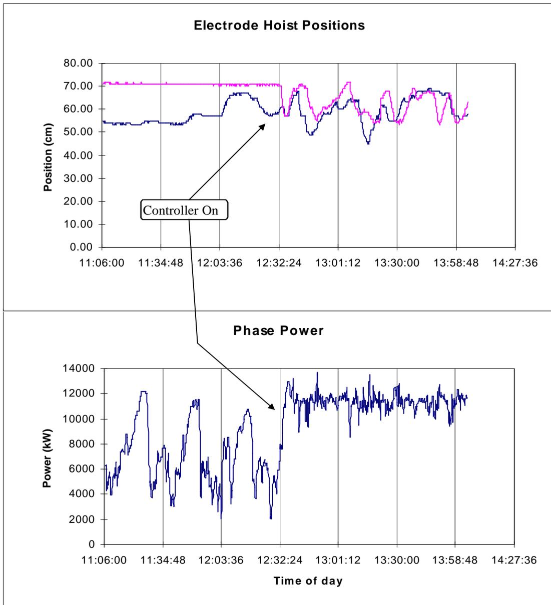
**Figure 7: Phase power without, and with control**
