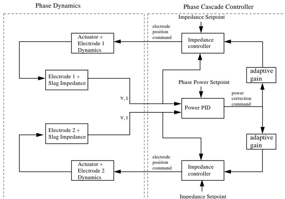
**Figure 8:** Cascade phase power controller for a six-electrode furnace
