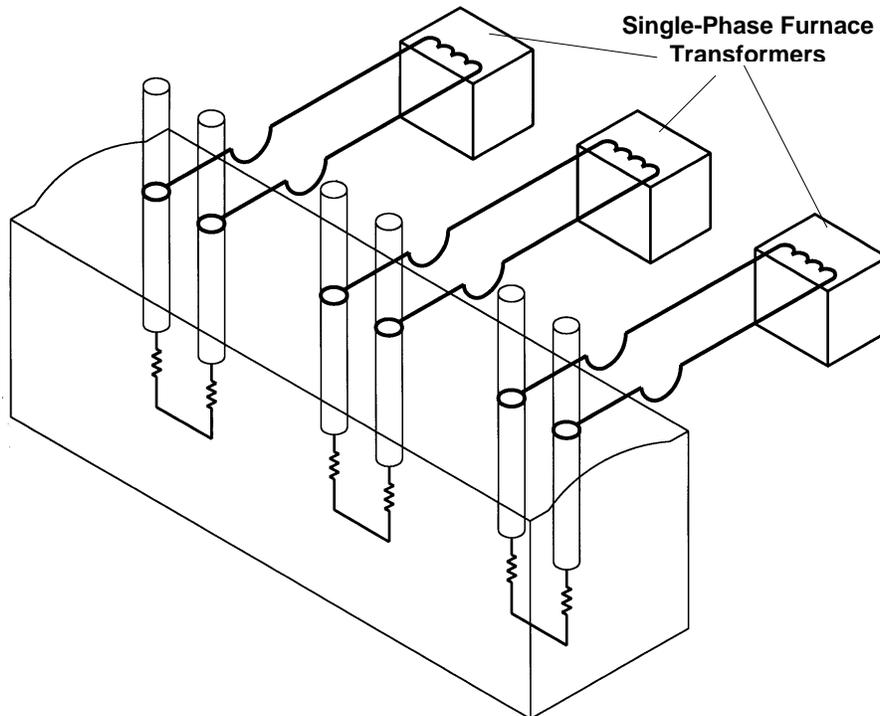
**Figure 5: Six-electrode furnace circuit diagram**
