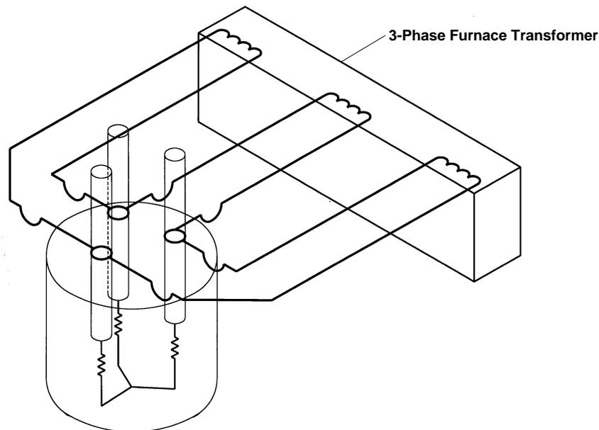
**Figure 2: Three-electrode furnace circuit diagram**
