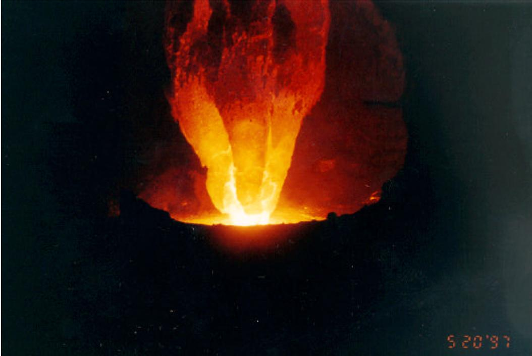
**Figure 3: Arcing electrode tip in a furnace**
