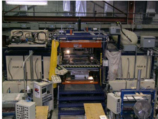
Figure 4: Monark Twin Sheet Thermoforming Machine
