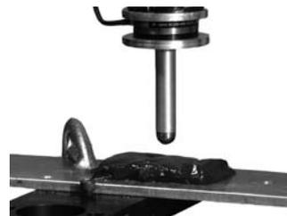
Fig. 8. Testing a well supported sample of liver.
