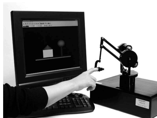
Note: The Phantom features a clever torque amplification capstan drive where only one cable is shared by two motors and provides for static balancing.
