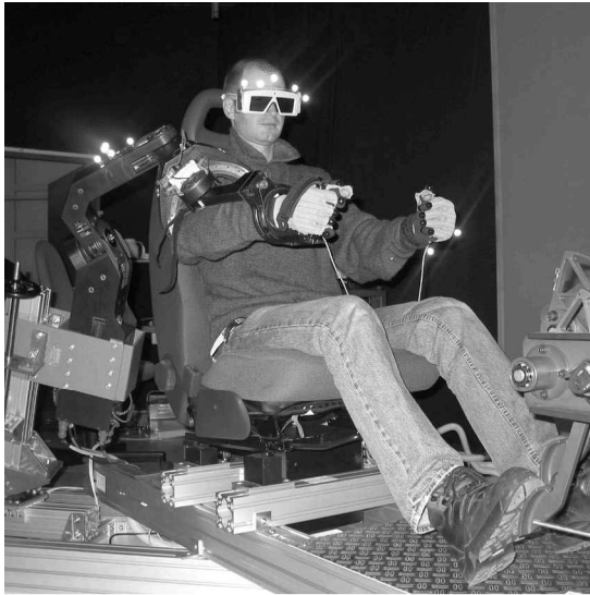
Note: The left panel shows such a device applied to the simulation of the driving experience for cockpit design optimization. The right panel shows a variant of this device accommodating two additional sub-devices able to simulate the manipulation of objects "out of thin air".
