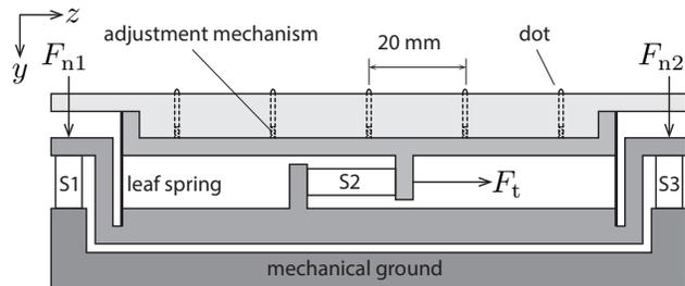
Fig. 1. The apparatus. The transducer measures the interaction forces of the finger exploring the Braille dot platform with dots of adjustable heights.
