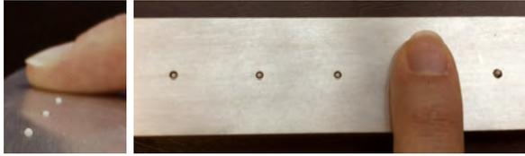
Fig. 2. The Braille dot platform consisting of five consecutive dots mounted on an aluminium plate. The finger had no inclination to the platform.
