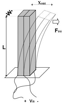
**Fig. 5.** Applying a differential voltage  $V_{in}$  between the middle electrode and the outside electrodes results in a lateral displacement  $X_{out}$  and a force  $F_{out}$  applied to the load at the tip of the bimorph. The bimorph has resonant frequency  $F_0$ . From basic cantilever mechanics, it is known that  $X_{out} \propto L^2$ ,  $F_{out} \propto W/L$  and  $F_0 \propto 1/L^2$ . Likewise, from basic electrical relationships,  $C_{piezo} \propto W \times L$
