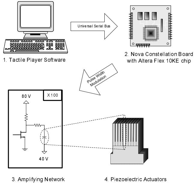
**Fig. 2.** The STReSS system is composed of four subsystems: A tactile player application (1) sends tactile images to the PLD (2). The PLD converts the tactile data into pulse width modulation (PWM) control signals used to drive a network of 100 switches (3). The switching amplifiers control voltages to drive the piezoelectric actuators forming the tactile array.
