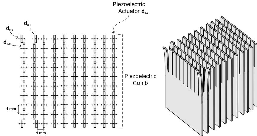
**Fig. 1.** Structural configuration of the piezoelectric actuator pack. Ten piezoelectric combs, each cut to form ten tooth-like actuators, are packed one next to another to form a matrix with one mm pitch in both directions. Four actuators are shown with an exaggerated displacement. The upper side is in contact with the skin.
