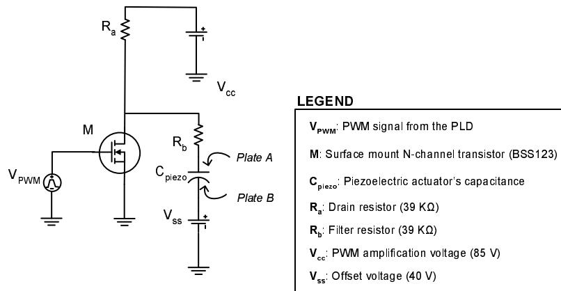
**Fig. 4.** An amplifying element comprises one transistor, two resistors and the piezoelectric actuator's capacitance. The 3.3 V PWMs are amplified to 80 V pulses before being filtered by the actuator. One of the piezoelectric's electrode (plate B) is offset by 40 V so that bipolar potentials of  $\pm 40$  V can be set across the actuator.
