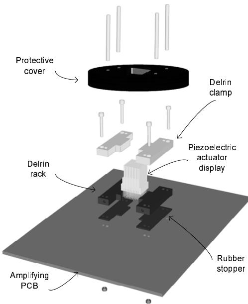
**Fig. 8.** A PCB supports one hundred amplifiers. The outputs are routed via an 8 layer board to a  $1 \text{ cm}^2$  pad having one hundred connections. The individual combs are held collectively using two racks and two clamps, forming 10 sockets.
