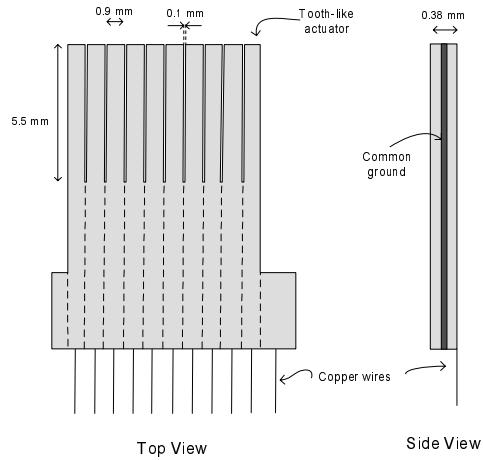
**Fig. 7.** Comb shape. Each tooth-like actuator is isolated from its neighbors by selectively removing the external electrodes. They all share the brass center shim as a common ground. Electric connections to the PCB are by small copper wires. Two shoulders are provided for clamping each comb in its socket slot. Sockets are made of two opposite racks attached to the PCB, as illustrated in Figure 8.
