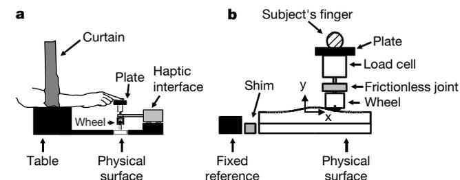
**Figure 1** Side (a) and front (b) views of the apparatus. Subjects pressed down on the manipulandum's plate and rolled it sideways ( $x$ -axis in b) to explore the shape of an interchangeable physical surface. The entire workspace was hidden from view behind a black curtain. The manipulandum was connected to a haptic interface (Methods) that operated silently.
