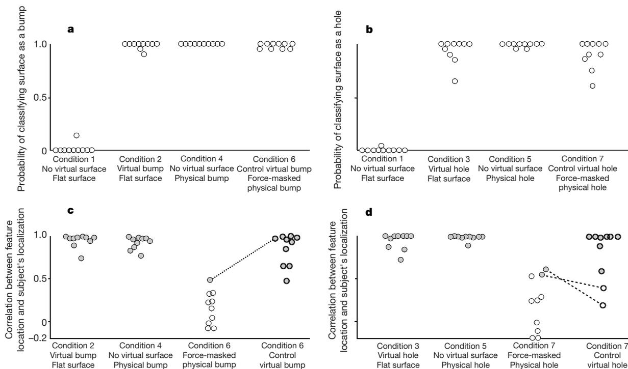
**Figure 3** Subjects used force to identify or locate shape features. Each symbol represents data from one subject. Subjects easily classified stimuli as bumps or holes when a virtual surface or flat physical surface combination was presented, or when virtual and physical surfaces coexisted, but not when a flat surface was presented alone (a, b). Subjects tracked the position of physical and virtual surfaces (c, d, conditions 2–5). However,
