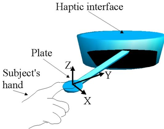
Figure 1. The experimental setup. Subjects pressed down on a manipulandum (plate) to interact with the haptic interface. The manipulandum is shown here positioned at the origin of our coordinate system, located at the center of the workspace.
