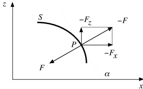
Figure 4. The forces involved in haptic exploration of a physical, frictionless surface  $S$ . Our LFFs can be related to  $-F_x$ , the lateral component of the normal force  $-F$  that the surface returns when a subject applies a force  $F$  to the surface.
