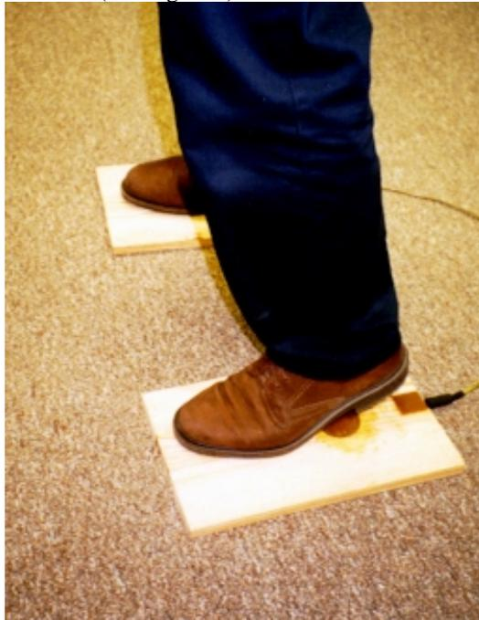
**FIGURE 7: foot-sensed vibrotactile stimulator**
