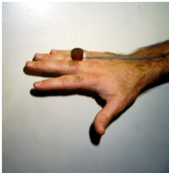
**FIGURE 6: ring-mounted vibrotactile stimulator**
