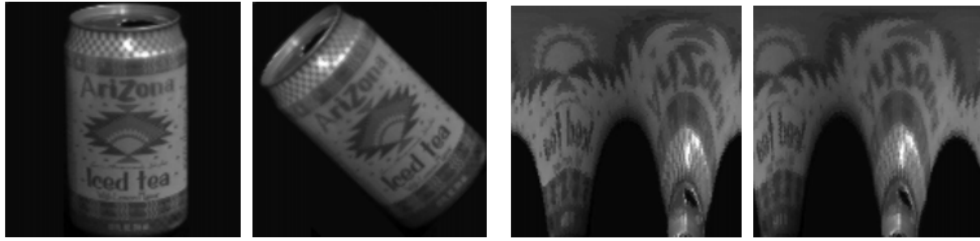
Figure 2: A sample image and its rotated version and their corresponding images in polar coordinates. We see that rotation corresponds to shift in polar coordinates. [Images taken from [3]]
