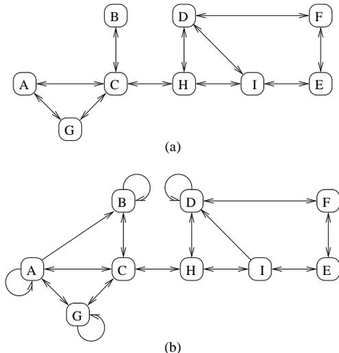
Fig. 4. Topological maps of the environment that were: a) analytically determined based on the layout; b) inferred by the algorithm;
