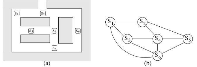
Fig. 1. An example of a sensor network which we wish to calibrate. a) The original ad-hoc deployment. b) The desired topological connectivity map of the network.
