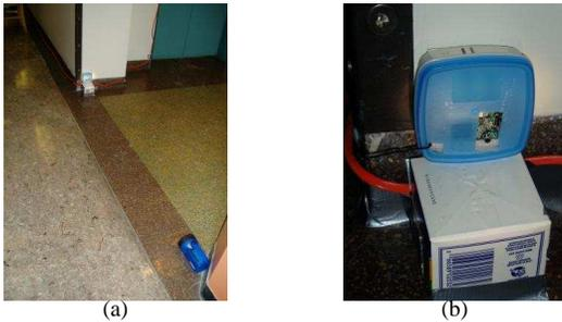
Fig. 2. a) Complete setup and, b) close up of a deployed photocell-based sensor constructed out of a flashlight and a Crossbow wireless sensor. (Plastic containers were used as protective covering during experiments.)
