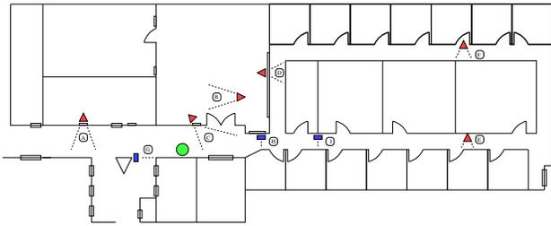
Fig. 3. The layout of the nine sensor (heterogeneous) network used for the experiment. Labeled triangles represent vision-based sensor positions (A-F) and labeled rectangles represent low-powered photo-based sensors (G-I). The circle represents the location of the central server.
