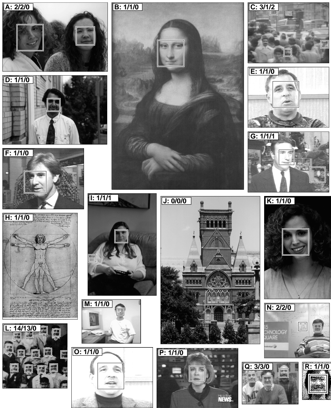
Figure 13: Output obtained in the same manner as the examples in Fig. 11. Some notes on specific images: Faces are missed in C (due to blurriness) and L (due to partial occlusion of the chin). False detections are present in C, G, and I. Although the system was trained only on real faces, hand drawn faces are detected in H and N. A, D, I, J, and K were scanned from photographs, B, H, and L were obtained from the World Wide Web, C, E, F, G, O, and P are digitized television images. M, N, and Q were provided by Sung and Poggio at MIT, and R is a dithered CCD image.
