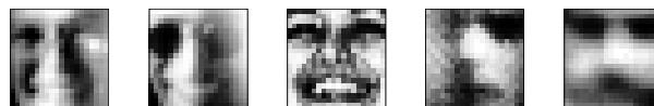
Figure 2: The steps in preprocessing a window. First, a linear function is fit to the intensity values in the window, and then subtracted out, correcting for some extreme lighting conditions. Then, histogram equalization is applied, to correct for different camera gains and to improve contrast. For each of these steps, the mapping is computed based on pixels inside the oval mask, and then applied to the entire window.
