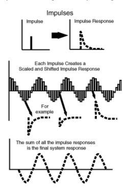
The way we use the impulse response function is illustrated in the above Figure. We conceive of the input stimulus, in this case a sinusoid, as if it were the sum of a set of impulses. We know the responses we would get if each impulse was presented separately (i.e., scaled and shifted copies of the impulse response). We simply add together all of the (scaled and shifted) impulse responses to predict how the system will respond to the complete stimulus.
