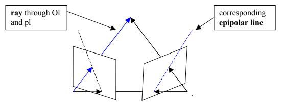
$\Rightarrow$  This allows us to restrict the search for the match of pl along the corresponding epipolar line. The correspondence problem has therefore been reduced to a 1D problem.
