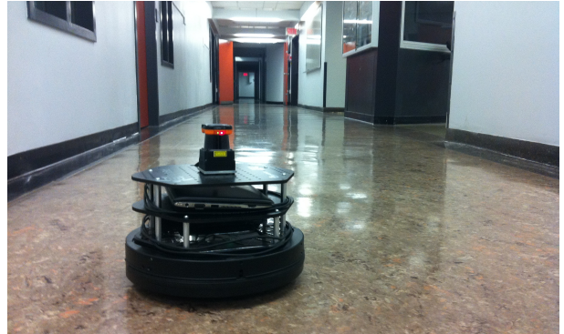
Fig. 1. The experimental setup used throughout this paper. The robot, a TurtleBot 2, is equipped with a Hokuyo laser range-finder used for navigation. The robot was used to explore the corridors of the Centre for Intelligent Machines, McGill University.
