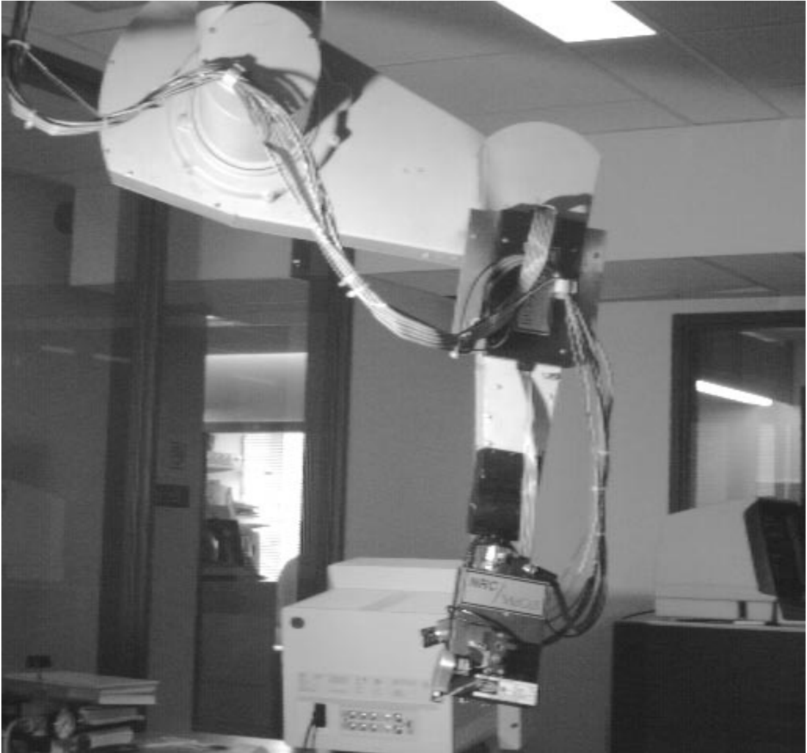
FIGURE 4.17. Active vision workcell at the McGill Centre for Intelligent Machines. A scanning laser range finding camera is affixed to the end effector of a PUMA 560 robot. A table directly beneath the robot base provides a suitable surface for scene objects, and also serves as the reference plane in our calibration process.
