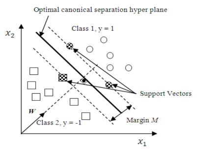
Figure 4-1: Illustration of two dimensional SVM model with separating plane represented by bold line and the two parallel planes with support vectors in the dotted lines.
