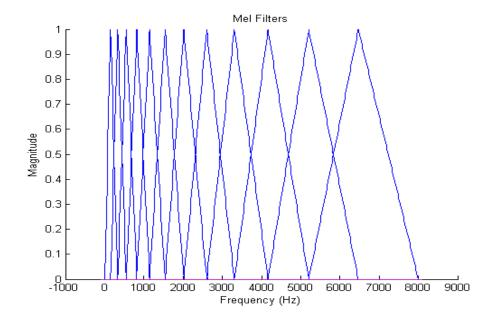
Figure 3-3: Bank of triangular filters used for Mel-Cepstrum analysis, given by:
