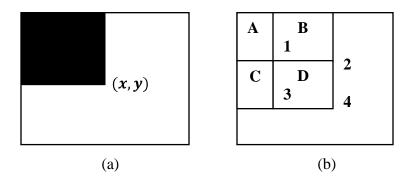
Figure 3-8: Integral image from Viola-Jones face detector. (a) Pixel location (x, y), contains the sum of pixels in the black shaded region. (b) The sum of pixels in D is  $(x_4, y_4) - (x_2, y_2) - (x_3, y_3) + (x_1, y_1)$ .
