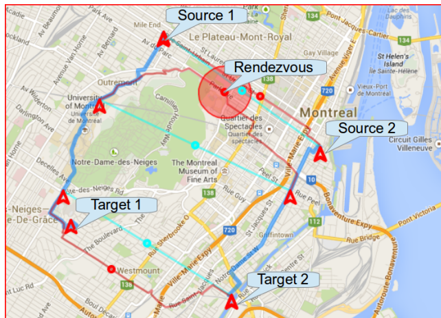
Fig. 1: Our rendezvous planner using Google maps API ©. The individual paths of the two agents are represented by the blue solid lines. Red arrow heads illustrate the waypoints. Small cyan and red circles indicate potential rendezvous points which are computed using Euclidean metric and actual travel times on the road network, respectively. The optimized rendezvous location using our cost function is shown by the center of the big red circular disk.
