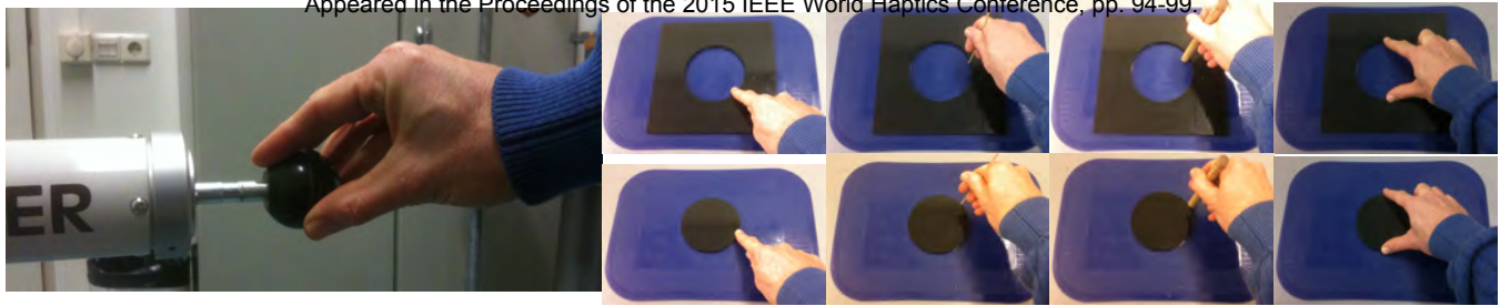
Fig. 3. The five conditions of the experiment: from left to right: the haptic device condition, the finger condition, the small probe condition, the large probe condition, and the bidigital condition. For the four conditions on the right: the top row shows the inside stimuli, while the bottom row shows the outside stimuli.
