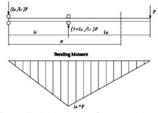
Figure 2. The bending moment of a two-support beam
