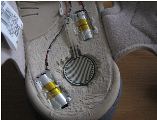
Fig. 2. A picture of one pressure sensor and two actuators embedded in the shoes.
