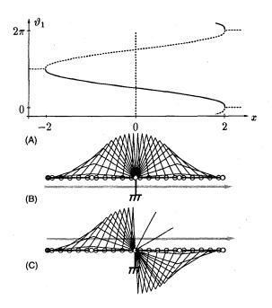
Figure 1: (A): Solutions of  $\vartheta_1$  (solid and dotted lines) for a planar 2R robot, with both link lengths equal to 1, following the x axis. (B): motion corresponding to the solid line solution. (C): motion resulting from switching solution branches (solid to dotted) using the self-motion singularity at the origin.
