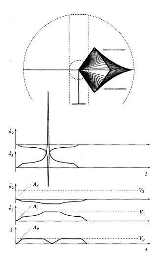
Figure 3: Motion out to and back from the PUMA workspace boundary. Upper plots show  $\dot{\vartheta}_2(t)$  and  $\dot{\vartheta}_3(t)$  when this motion is done at constant speed. Lower plots show results after algorithm time scaling has been applied. By changing configurations at the singularity, it is possible to maintain a finite joint speed while transiting the singularity, even though the speed along the path (indicated here by  $\dot{s}$ ) is brought to 0.
