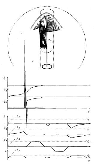
Figure 4: A parabolic motion taking the PUMA to the triple singularity near the ready position. Upper plots show  $\dot{\vartheta}_1(t)$ ,  $\dot{\vartheta}_3(t)$ , and  $\dot{\vartheta}_4(t)$  when this motion is done at constant speed. The extremely large spike in  $\dot{\vartheta}_4$  is due to the self-motion at the wrist singularity. Lower plots show results after algorithm time scaling has been applied.
