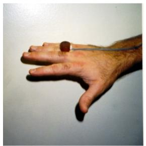
FIGURE 6: ring-mounted vibrotactile stimulator
