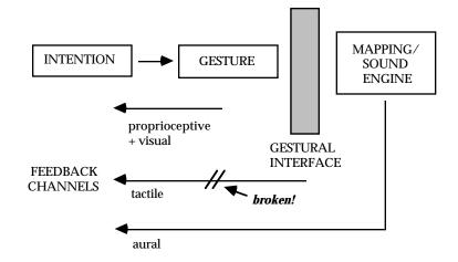
**Figure 1: Performing with an open-air controller** In systems which track a performer's gesture through remote sensing technologies—such as infrared, ultrasound, or video—the tactile feedback loop is broken, forcing performers to rely on proprioceptive, visual and aural cues.
