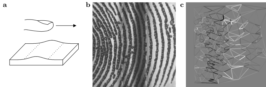
Fig. 7. a) A finger slides on a ridge of millimetric scale (0.5 mm high). b) The skin is imaged and its anatomical features tracked. c) Regions of skin compression are represented by darker segments, while regions of stretch have lighter segments [7].
