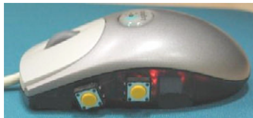
Figure 5: Vibrotactile mouse used to display the haptic icons used in the turntaking protocol. Two buttons were added to the side, to enable special protocol features; such buttons were available in other mice at the time, but not the vibrotactile one.
