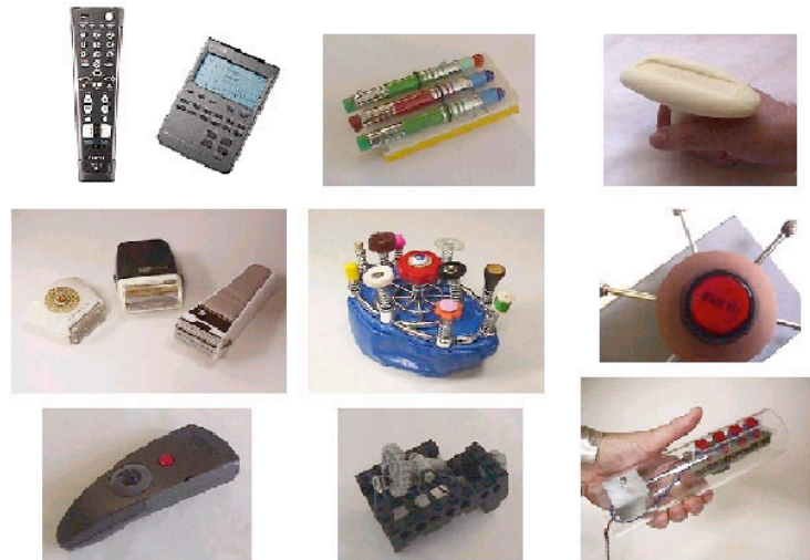
Figure 3: Early prototype for the handheld media controller project. Found objects and state-of-art examples, Lego + rubber band transmissions, whimsical and serious non-functioning concepts, and narrowly targeted functional engineered prototypes.
