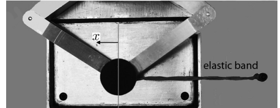
Fig. 7. Experimental Apparatus. The pre-tensioned elastic band allows repeatable wall contact with a passive operator.
