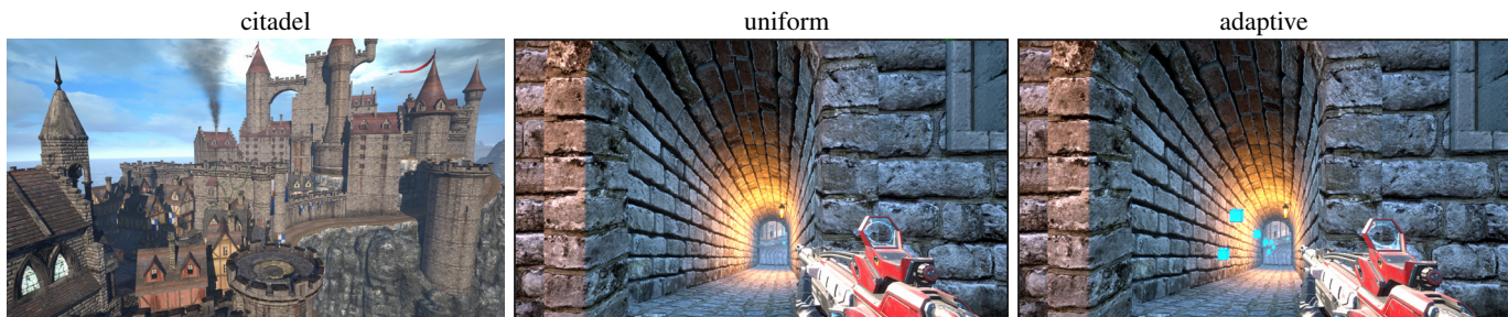
Fig. 12. Narrow tunnels and corridors are common in complex game scenes such as EPICITADEL (left). Uniform sampling (middle) can miss such regions entirely. Runtime decoding will fail as the player enters such an area, causing unbounded rendering errors. Increasing global sampling resolution to about a meter resolves the issue but makes the precompute and memory cost impractical in such large game scenes. Our technique (right) adapts resolution locally to guarantee sampling within thin features avoiding such errors. Probes shown with blue boxes.
