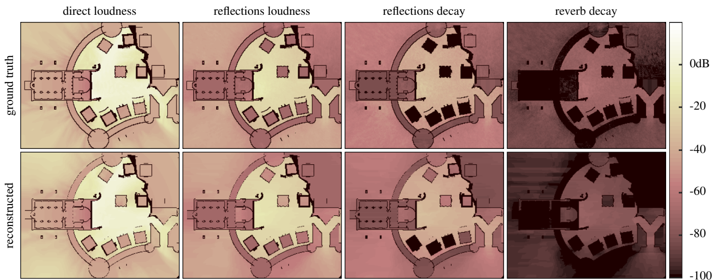
Fig. 10. Reconstruction accuracy for all parameter fields on EPICCITADEL.
