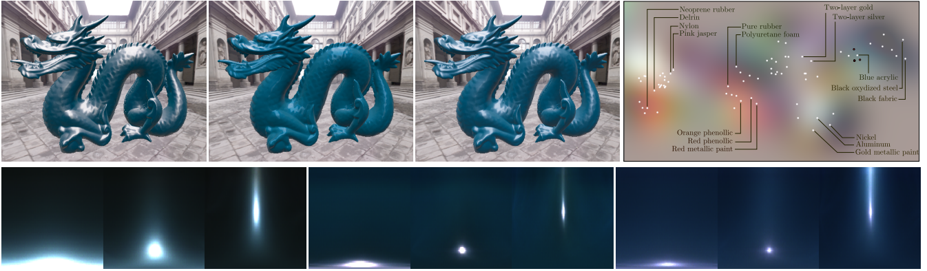
Figure 10: Real-time exploration of our BRDF manifold. 3 materials (circle points) are picked up in the vicinity of blue-acrylic, by clicking in the 2D latent space (top right), showing consistent local variations of both color and shininess. Here latent variables were optimised using all 100 materials of the MERL database. The dragons are screenshots from our real-time rendering (25 fps) prototype, which shades interpolated materials along with all combinations of dynamic geometry, view points and lighting (see sec. 5.1) using zonal harmonics up to L = 40 [SBN15]. The slices of the interpolated BRDFs are also visualised. A live demonstration is presented in our video.
