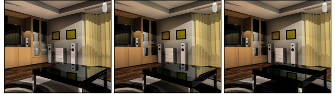
Figure 19: The number of probes primarily affects diffuse inter-reflection quality. From left: 1 \times 4 \times 1 , 4 \times 4 \times 4 , 8 \times 4 \times 8 .
