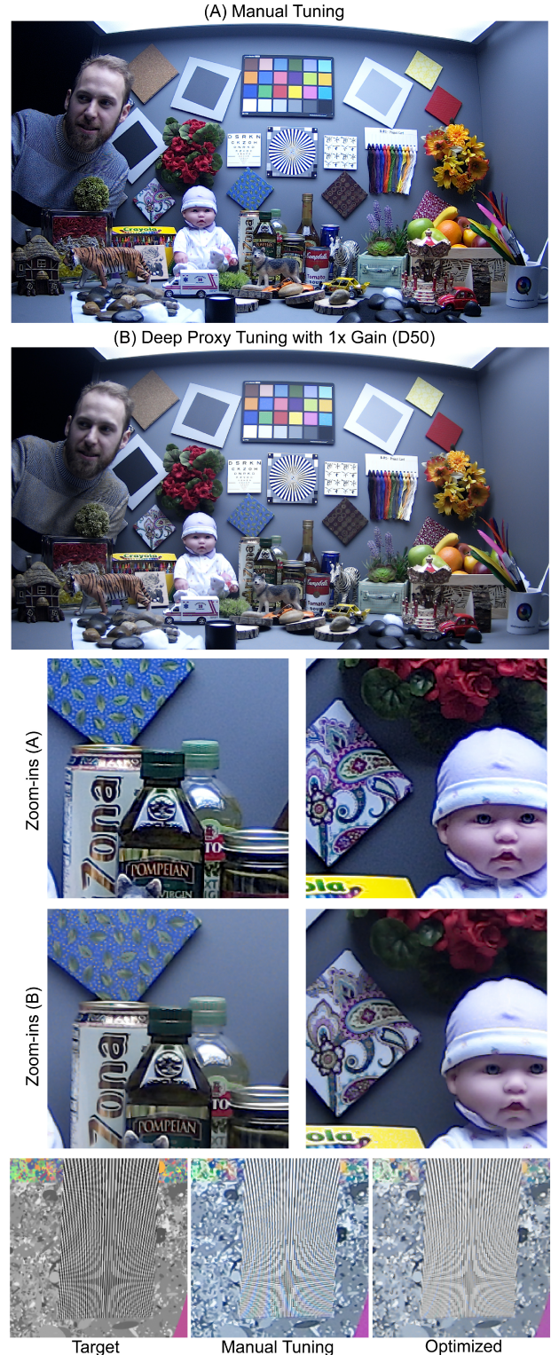
Fig. 10. Low-noise imaging example. This example demonstrates that the current approach achieves golden-eye tuned parameters which required months of manual optimization. The bottom inset examples visualize the improvement in color moire, measured in Table. 3.
