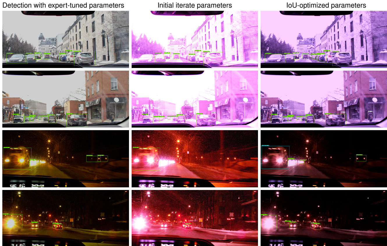
Fig. 12. Qualitative object detection results. While the images produced by an ISP with expert-tuned parameters (left) may look more natural to the human eye, the performance of a pretrained object detector can be improved by adjusting the ISP parameters to maximize the intersection-over-union score (IoU) of the detector (right). The middle column shows the detection results with the initial tuning parameters.
