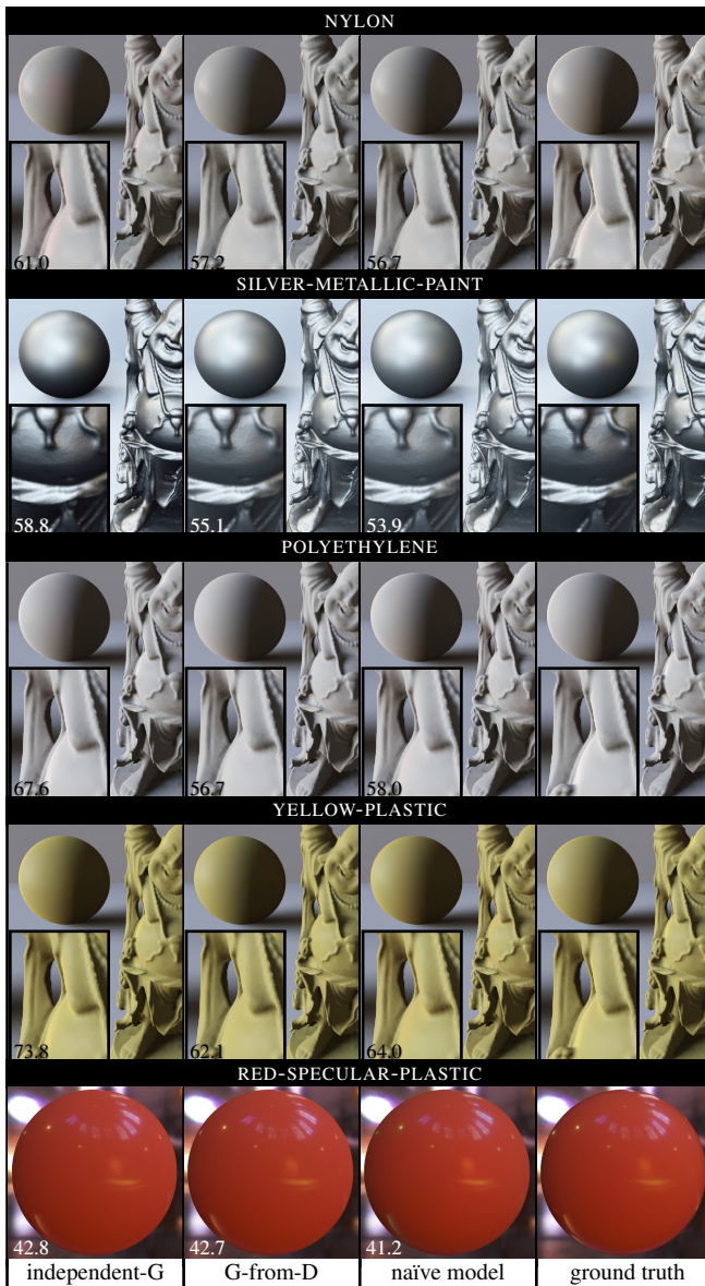
Fig. 9. Rendering comparison for non-parametric fits (close-up in the inset). PSNR over the image is displayed in the lower left corner. The independent-G method better preserves backlighting effects (NYLON and POLYETHYLENE), darkening (SILVER-METALLIC-PAINT), highlights (YELLOW-PLASTIC), and avoids color-shifting (green shift in highlights of naïve rendering for RED-SPECULAR-PLASTIC).
