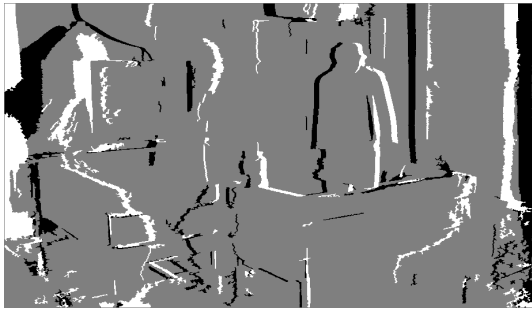
Figure 5. The half occlusion regions detected by our approach. Black regions are the left-half-occlusions and white regions are the right-half-occlusions. The two half-occlusion maps are overlaid onto a single image for ease of display.
